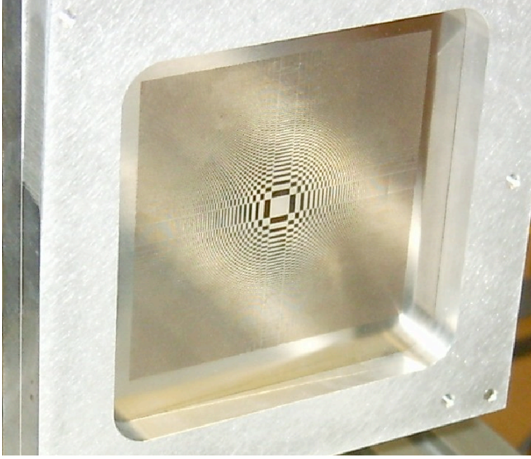
Fig. 4 80 mm square Fresnel primary array carved into a thin 80 \mu\text{m} stainless steel foil, used for optical tests. (58 Fresnel zones, 26 680 subapertures).
